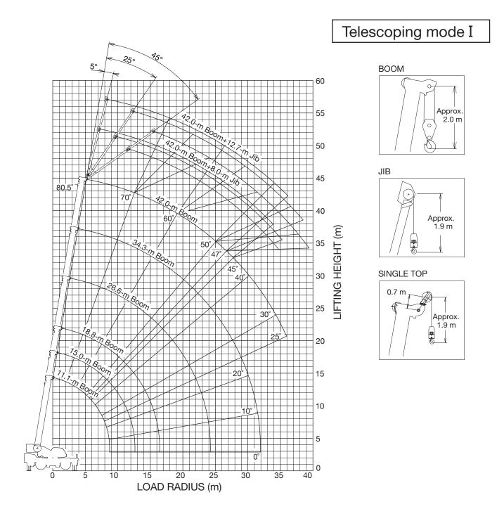
The above lifting height and boom angle are based on a straight (unloaded) boom and machine standing level on firm supporting surface. Allowance should be made for boom deflection obtained under loaded conditions. The above working range is shown on condition with outriggers fully (7.0 m) extended.
